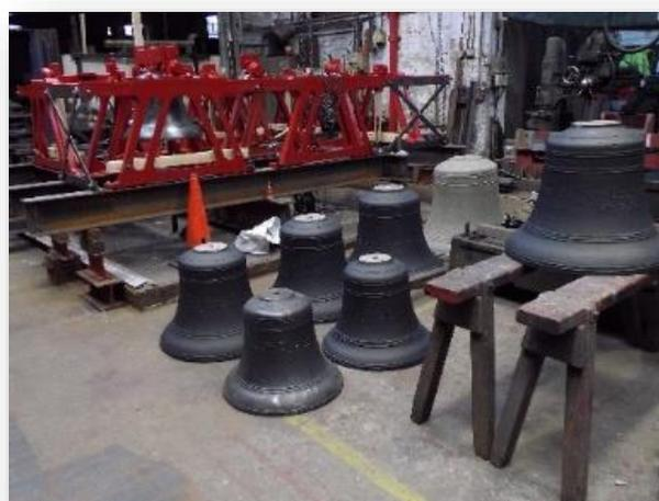
*The completed installation being set up at the Loughborough foundry for testing.*
